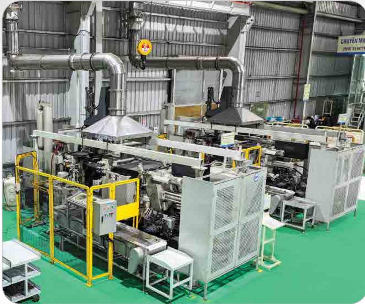
**ALUMINUM CASTING MACHINING LINE**
