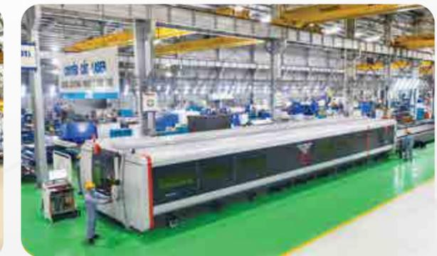
**SHEET STEEL LASER CUTTING MACHINE**
