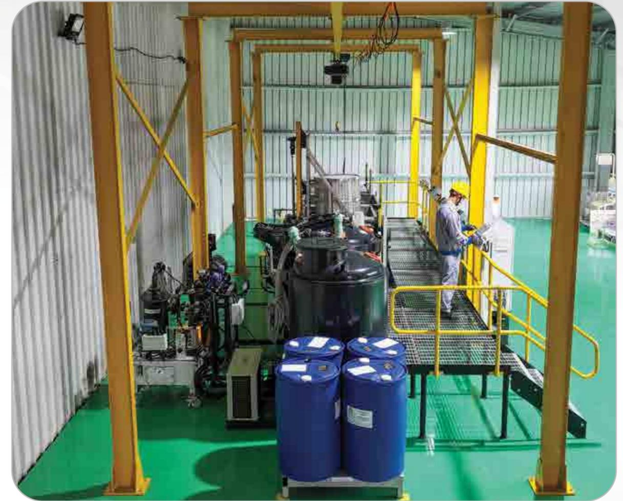
The vacuum impregnation system is a specially designed system for impregnation under vacuum pressure conditions.
