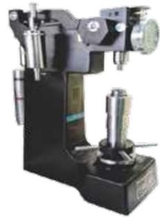
Material hardness testing machine
