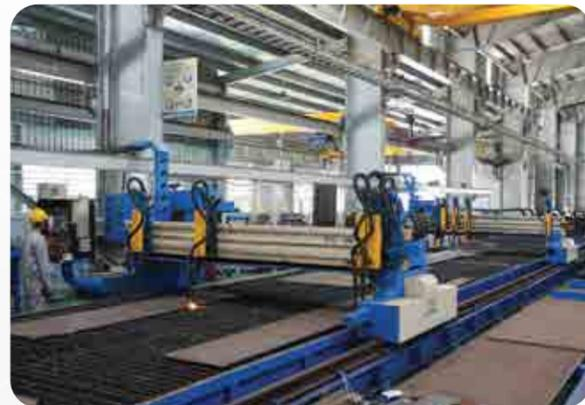
**CNC OXY-FUEL AND PLASMA CUTTING MACHINE**
