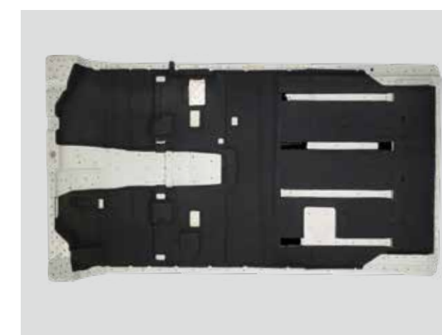
JIG cắt tap-pi sàn xe KIA KA4 KIA KA4 floor carpet cutting JIG
