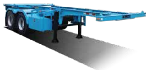
20', 2 trục, 4 khóa gù 20 feet, 2 axles, 04 twist locks
