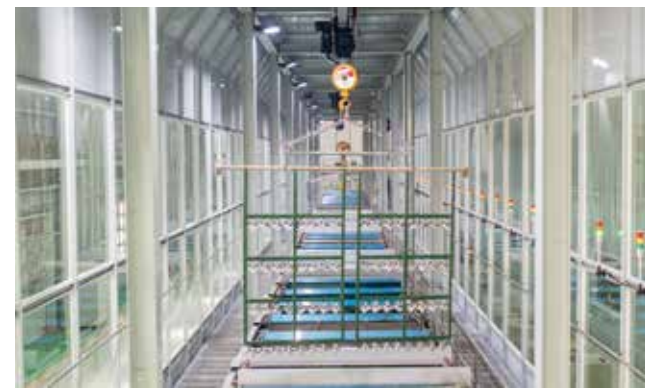
ZINC-ELECTROPLATING LINE Load: 150 kg Axis travel: 1,800 x 1,400 x 400 mm
