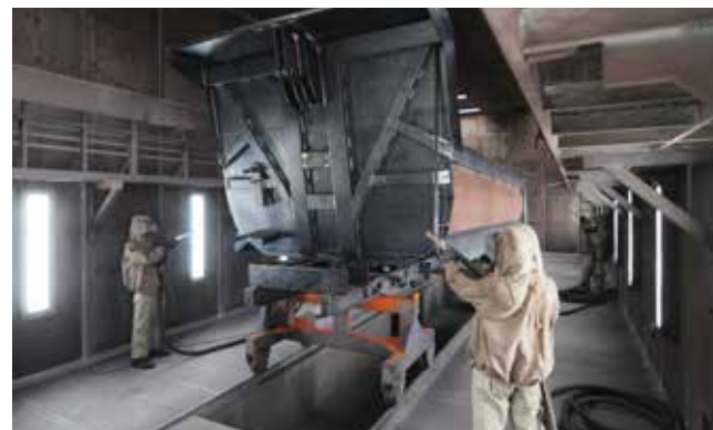
SHOT BLASTING BOOTH Load: 10,000 kg Max material size: 14,000 x 2,500 x 3,500 mm
