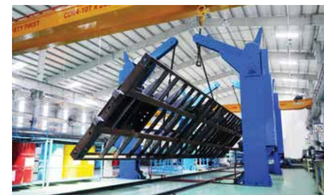
SEMI-TRAILER CHAIN TURNING EQUIPMENT Max load on table: 10 tons Dimension: 6,000 x 4,100 x 5,000 mm
