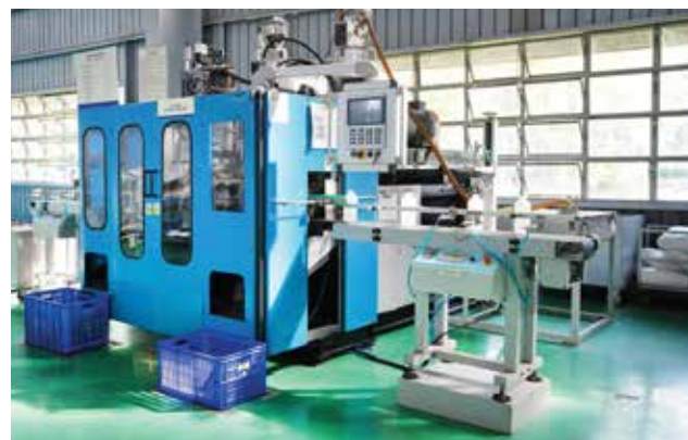
EXTRUSION BLOW MOLDING MACHINE 0.5~5L
