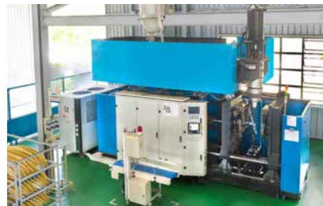
EXTRUSION BLOW MOLDING MACHINE 10~30L
