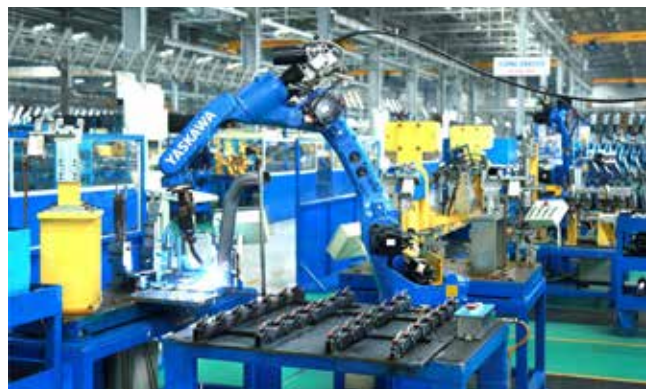
WELDING ROBOT LINE Quantity: 100 machines Gas metal arc welding Flux cored arc welding
