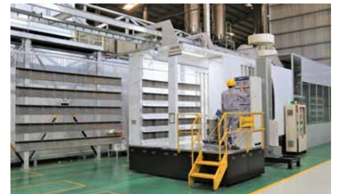
POWDER COATING LINE Load: 140 kg Max material size: 5,500 x 2,000 x 600 mm
