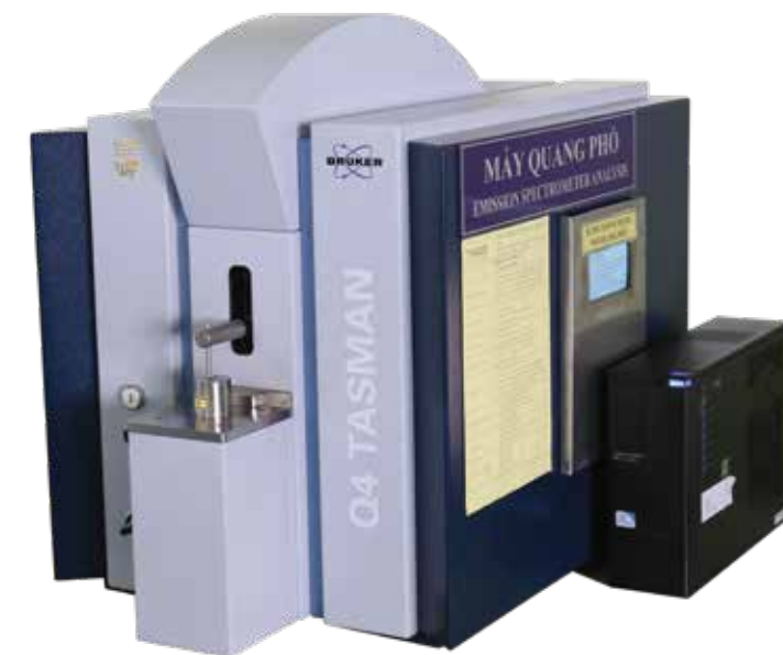
Spectrograph machine (material composition testing)
