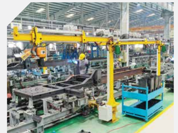
3 Welding to connect chassis frame
