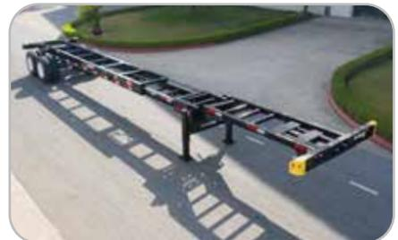
Cross member linked chassis structure can stand high bending force
